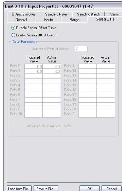
Figure 7.4: Setting a 22-Point Curve Using Wireless Instrumentation Manager
