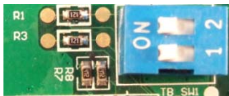
Figure 11 The Biasing Resistors and Termination Dipswitches (IPS-101/201)
