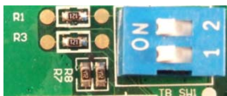
Figure 12 The Biasing Resistors and Termination Dipswitches (IPS-102/202)
