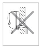
The hose must NOT slant upwards.
