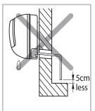
Keep a clearance of at least 5cm between the end of the hose and the ground.
