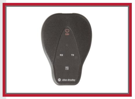
**Modbus RTU Pass-Thru Support** – The module can also be configured to operate as a RS-232 (DB-9) to RS-485 (RJ45) serial converter, where Modbus RTU messages pass-thru both directions in the module.
