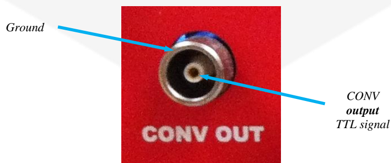
Figure 6 – CONV output connector
