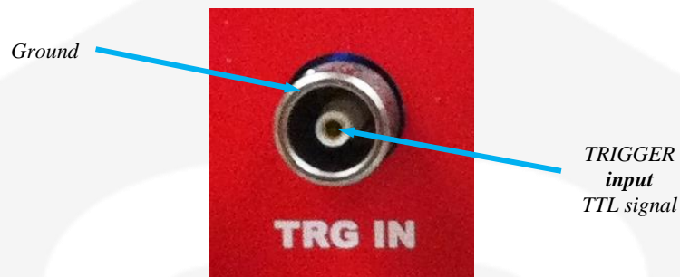
Figure 5 – Trigger input connector
