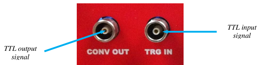
Figure 4 - I/O Interface Connector
