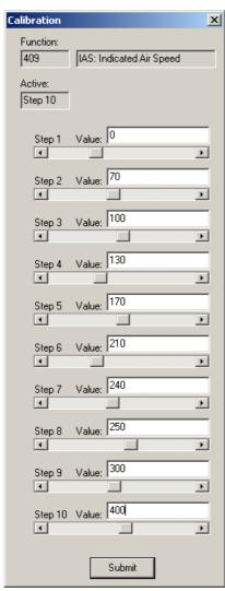
This example uses a 450 knots Airspeed indicator scale as used in an Airliner.
