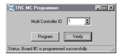
**Note:** the field Multi Controller ID does not necessarily tell you the correct number of the Multi Controller when using the "verify" function, only the status line does!
