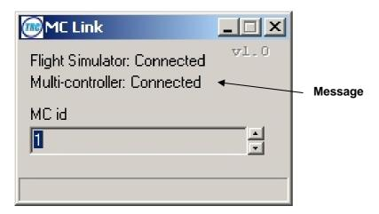
The MC Link window also tells you when the Flight Simulator software is connected, when the Multi Controller is connected, or when the ID is already occupied. The MC Link ID field always defaults to the number one (1). Therefore, if you have previously connected a Multi Controller with an MCLink, at the startup of the next one, the message "Already Occupied" will be displayed, meaning that you have to select a different number. The possible messages are:
