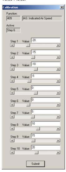
Always start to calibrate clockwise. This means that you must enter the lowest (or most negative) value in the first field and then the next higher (or less negative) value in the subsequent fields.
