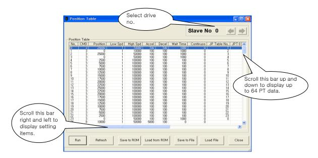
Position table data can be changed at any time. The position table can save up to 64 step data. If the position table is used to the program area, it may be used for all point numbers without restriction. That is, it is possible to start at a random point number and jump to other point number.
