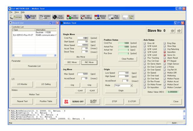
This is the basic window to operate the program. Each window is displayed in this window. The user can open each window with a toolbar.
