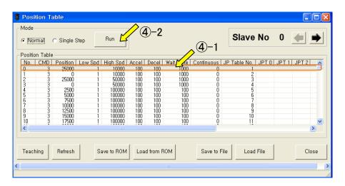
While PT No is operated in sequence, PT lines in service are changed in grey. Also, the user may monitor the operation status as described at '7.3 Position Status' and '7.4 Axis Status' through 'Motion Test' window,
