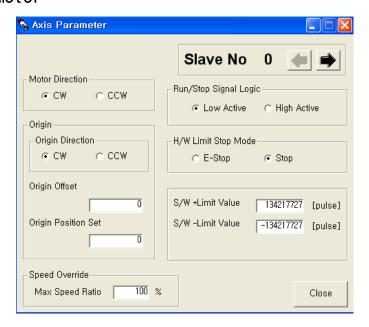
The above window is to enable the user to easily operate some important items of '3. Parameter List' items according to each function.
