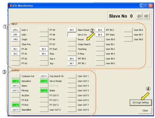
I/O Monitoring of Version 8 level GUI
