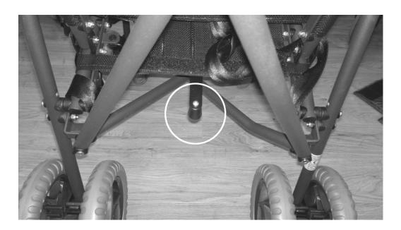
The image above shows the seat locking lever. When unfolding the buggy this must be pushed fully forward.
