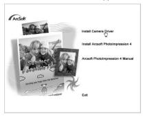
Click on *Install Camera Driver*. A setup wizard will guide you through the driver installation process. When its finished click *Finish* when prompted – this will restart your computer and complete the driver installation process.
