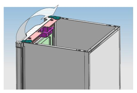
$B_{\, \times}\,$  replace the door bearing bush and the limit block.
