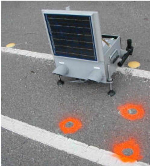
count, speed, volume, and classification for up to four lanes with traffic moving in one or both directions. The device is designed to handle all types of traffic, that is, freeways, arterials, collector and local street traffic, as long as the pavement is sufficiently flat. The beams are sensitive to ORADS placement and highway drainage sloping (road crown).
