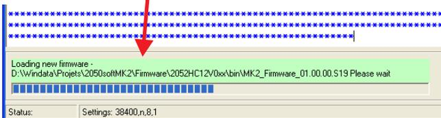
After few minutes you will have a message box saying that the upload is done. Set the rotary switch back to 0 then press the reset button. Your 2050 System is now running with the new firmware. You can close your Configurator program at this point.
