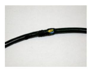
la Damage to power cable sheath
