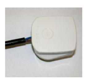
3b Inadequate strain relief
