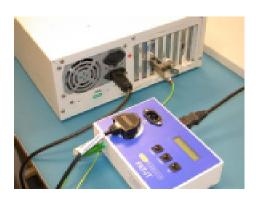
PAT-IT automatically assesses the test result for a pass or a fail.
