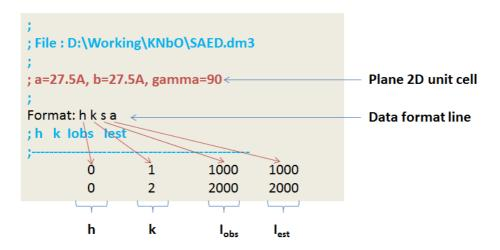
**h** and **k** are is for h and k 2D Miller indices, **s** and **a** are for the observed and estimated intensities. Each data line should contain single reflection information. The content of each data column is explicitly described by the "**Data format line**".
