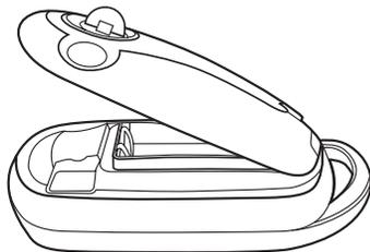
3. Install two AA batteries as shown.
