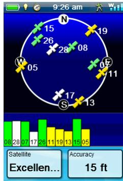
The Satellite Status screen displays a graphical representation of the satellites overhead in relation to you current location (the centre of the circle). The colour of the satellite graphics, as well as the bar graph, indicate the signal strength of the signals being received. The numbers indicate the assigned satellite designation. The data fields at the bottom of the display are customisable (see *Customising the Data Fields*).
