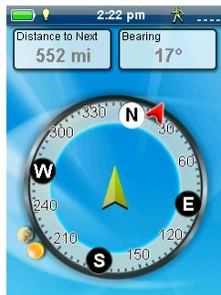
The Compass screen displays a recognisable compass that can be used to display your heading and your heading's relation to the sun, moon and your destination (red arrow). The data fields at the top of the display are customisable (see *Customising the Data Fields*). The graphic displayed that is used for the compass is customisable as well.
