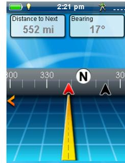
The Road screen displays a graphical road with a strip compass above the road. This compass displays your heading and your heading's relation to the sun, moon and your destination (black arrow) when they are within 50 degrees on either side of your heading. The data fields at the top of the display are customisable (see *Customising the Data Fields*).
