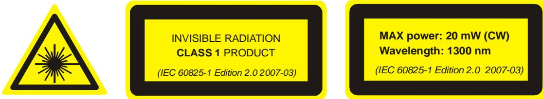
**FIGURE 1.5.** Warning Labels for Class 1 Laser Products.
