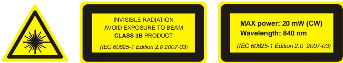
**FIGURE 1.8.** Warning Labels for Class 3B Laser Products.
