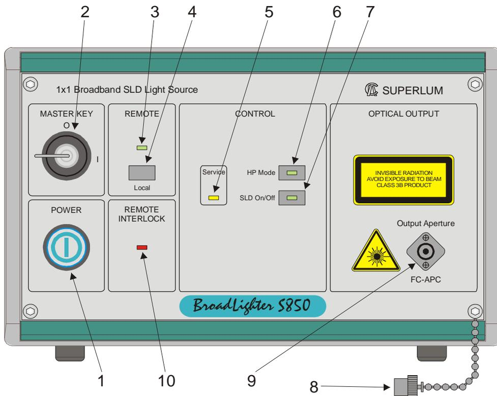
**FIGURE 3.1.** Front-Panel Features of the BroadLighter.
