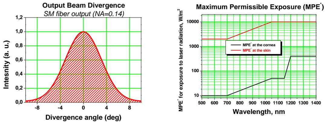
**FIGURE 1.6.** Examples of the Output Beam Divergence and the MPE.
