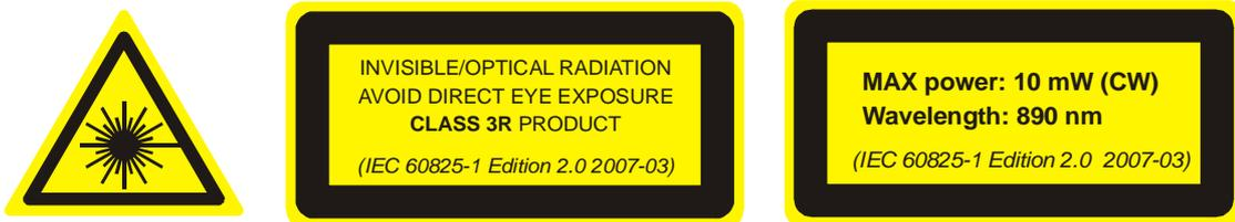
**FIGURE 1.7.** Warning Labels for Class 3R Laser Products.
