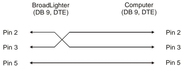
**FIGURE 4.1.** The Wiring Configuration for RS-232 Communication.
