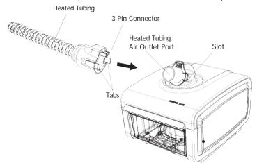
Note: Non-heated Philips Respironics tubing (15 or 22 mm) can still be used with this humidifier with the heated tubing air outlet port. Simply connect the tubing to the air outlet port. Refer to the therapy device manual for setup instructions.
