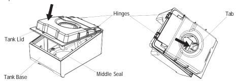
Note: If the lid does not close easily onto the base, separate the two parts, reassemble the tank, and inspect it again. CAUTION: Do not fill the water tank above the maximum fill line. Damage to the humidifier or therapy device may occur. If the water tank is overfilled, water may leak out of the tank inlet (located on the back of the tank) when installing the tank lid.
