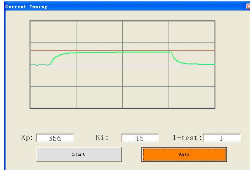
Figure 24: Kp=356, Ki=15 (poor performances)
