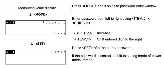
If the password is wrong, [FAIL] is displayed and it returns to the password entry window.
