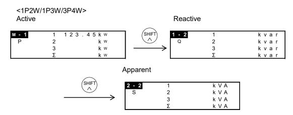
•Eco-POWER METER displays the power as below.
