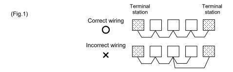
◆How to connect KW2M-A (2-wire) and KW9M (3-wire)
