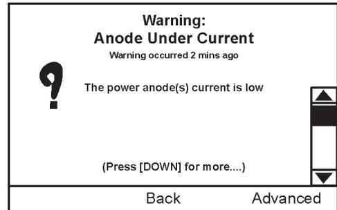
• **Faults:** This is a safety related condition that has been detected by the heater.
