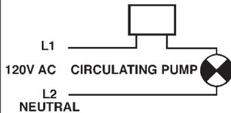
WIRING DIAGRAM FOR BOILER TO TANK LOOP
