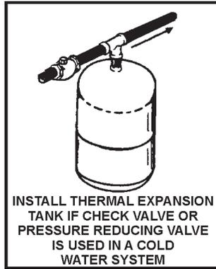
INSTALL THERMAL EXPANSION TANK IF CHECK VALVE OR PRESSURE REDUCING VALVE IS USED IN A COLD WATER SYSTEM
