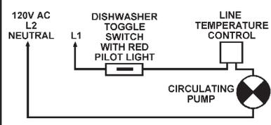
WIRING DIAGRAM FOR
