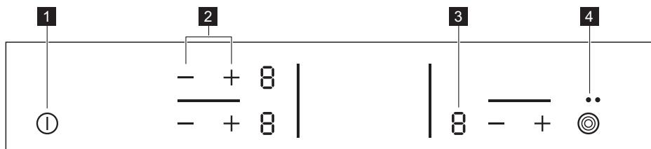
**Use the sensor fields to operate the appliance. The displays, indicators and sounds tell which functions operate.**
