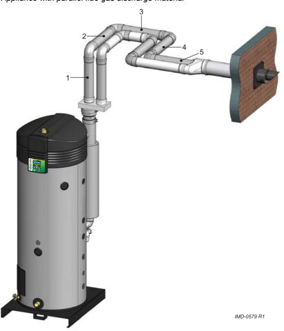
The longest pipe must be used to check the maximum length. In this case, the chimney pipe is the longest. This is 25 metres. This 25 metres is the sum of pipe sections 1, 2, 3, 4 and 5. The length of the transition piece can be ignored. The total number of bends used *in the chimney flue and air supply* is 8. The bend in the transition piece can be ignored. According to the table, 4.6 metres per bend must be added. This brings the total pipe length to:
