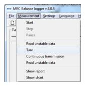
The scale will display  ${\bf 0}$ , and all performed measurements will be of net value.
