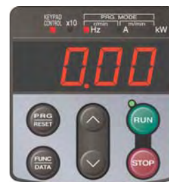
Figure 5.2 Display of the LED Monitor after Power-on
