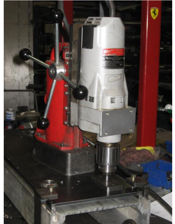
Figure 3: Hole Sawing Back structure
