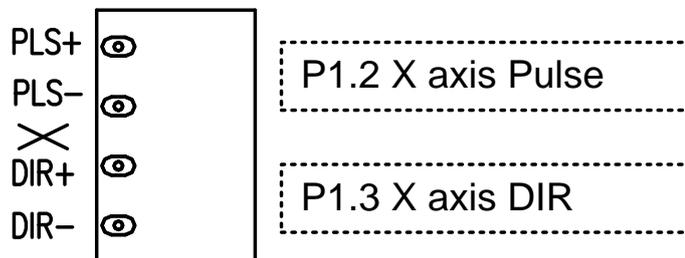
This is the port to join the driver in each axis and is made by Pins above. This port can link with revolving axis as well as moving straightly in each axis and can do also speed control for by connecting to motor driver for spindle.
