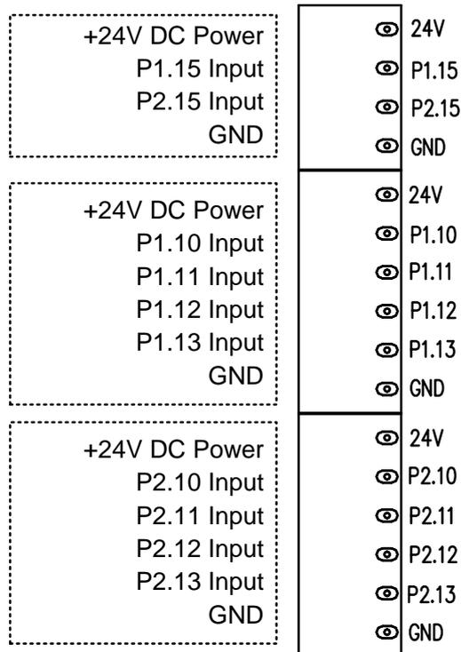
There are total 10 connectors (5 for port1 / 5 for port2) as above picture, It has each 4 or 6 pins. 24V Pin here provides power of exterior sensor and can be joined to the sensor to be input by +24V
