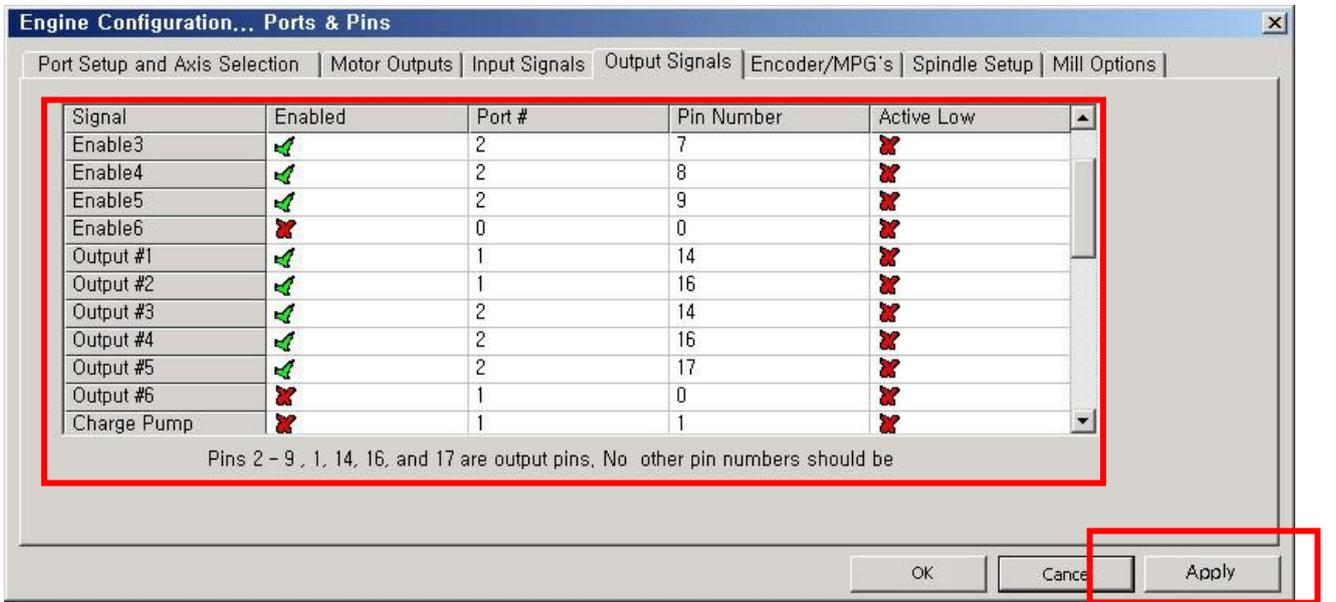
Enable 2~5 is the pin assigned by Open Collector Output.
