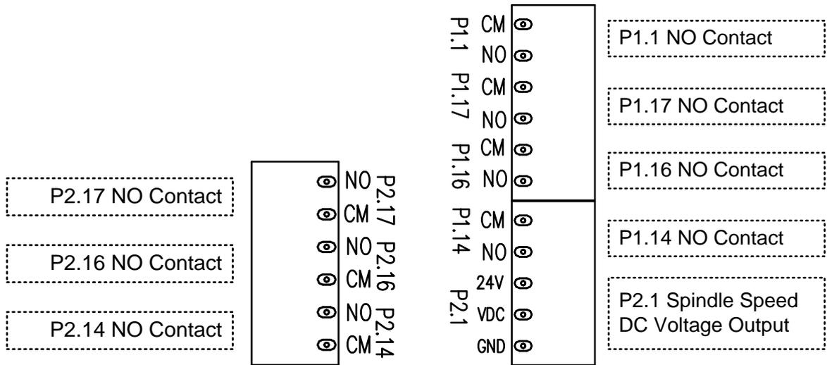
This port outputs 0~5V or 0~10V DC voltage for speed control of spindle. In Mach3, it is outputted after the PWM signal is converted to DC voltage when speed control of spindle by PWM mode.
