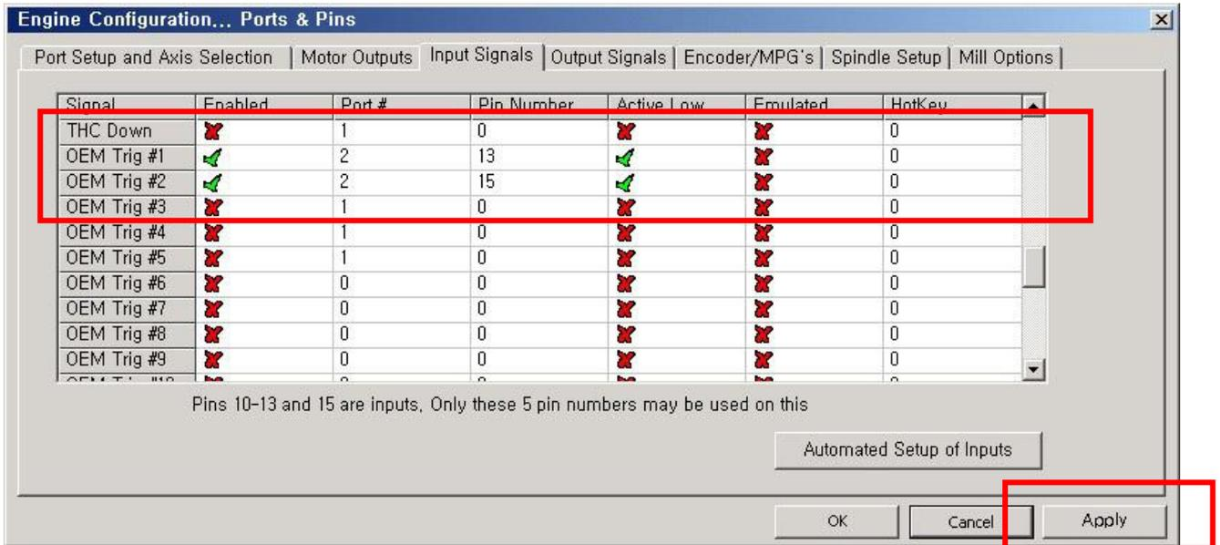
For OEM Trigger #1 & #2 are assigned for Cycle Start and Feed Hold button.
