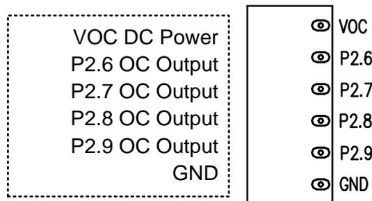
It is assigned 6,7,8,9 in Port2 and can join motor driver & can link with the relay for exterior control too.
