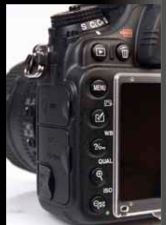
Replay function buttons double as short-cut keys to the main capture adjustments for ISO, white balance and image quality. The button with the paintbrush icon accesses the 'Retouch Menu' in replay mode or the 'Picture Control' presets in the camera's capture mode.
