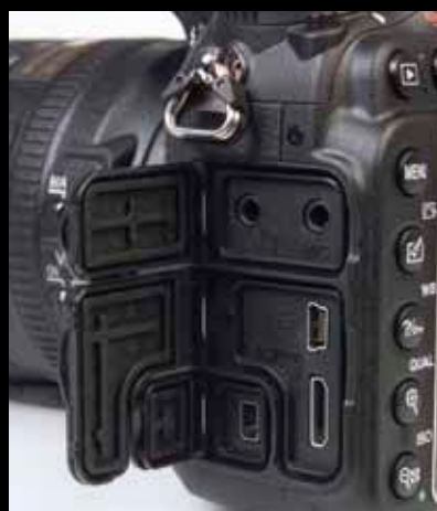
The D600 delivers an uncompressed video feed to its HDMI output and has both a stereo audio input and an output.
