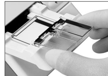
8. **DO NOT PUSH IN THE DRAWER.** Press **RUN**. The drawer will close. During the test, the screen will display:
