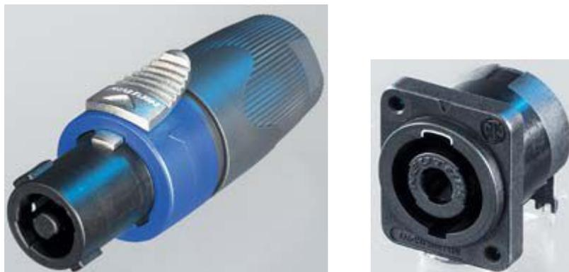
Heavy gauge wire should be used for the speaker cable between your bass amplifier and the external Speakon plug for the high currents that may go to the bass drivers. One bass amplifier + & - output should be connected to terminals 1 + & - of the Speakon plug (which are connected by the Kumbar Speakon socket to one bass driver); likewise the other output to terminals 2 (shown here in rear view):
