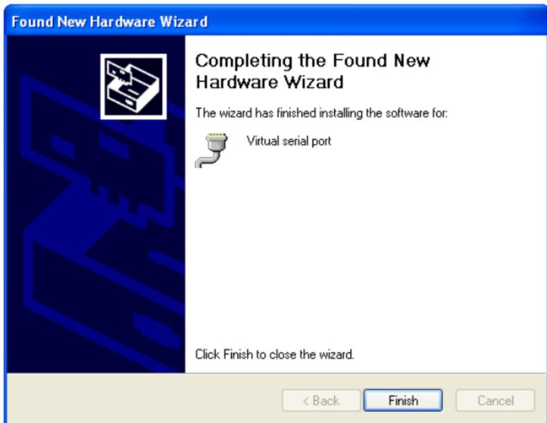
8. The Virtual COM port activates automatically when the printer is switched on.
