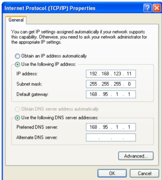
**Assign the IP address of the Host PC
