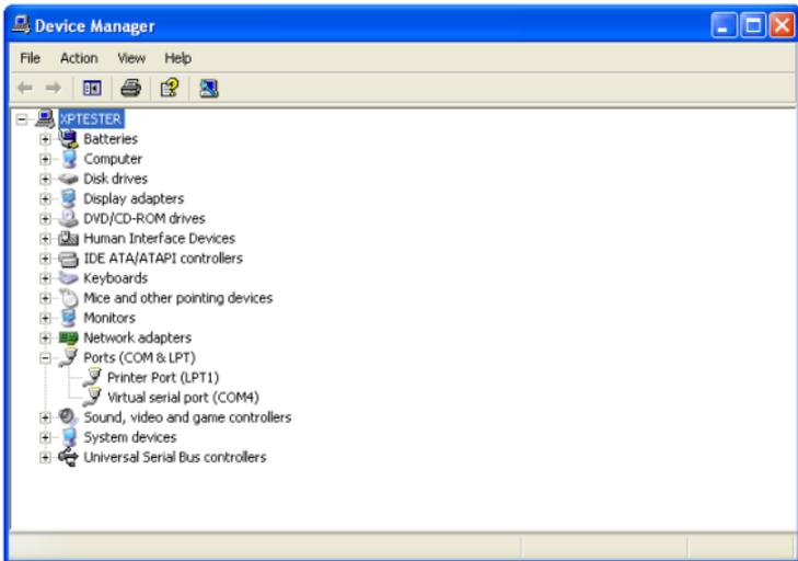
When turn on the printer, the Virtual COM activates automatically (Virtual Serial Port).
