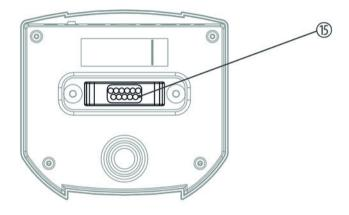
15 Multiple socket for connecting the pads.
