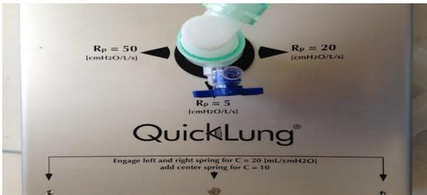
It should be used with both leak settings in the OFF position. Air will escape otherwise.
