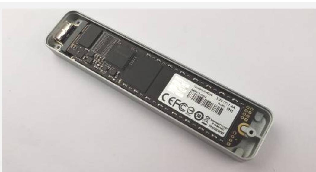
**6** Make sure your JetDrive and USB to SATA adapter is laying flat inside the enclosure
