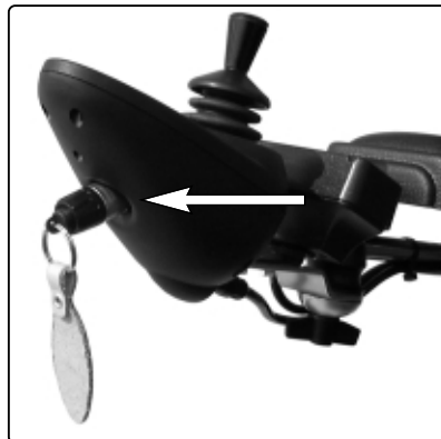
Fig. 13. Panel outlet with security key
