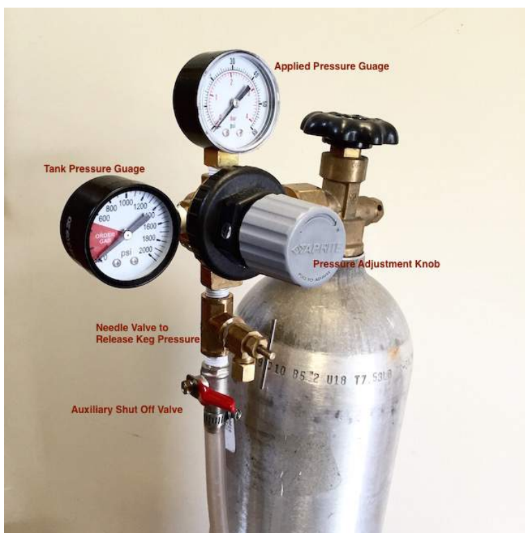
Proper setup of a CO2 pressurizing tank
