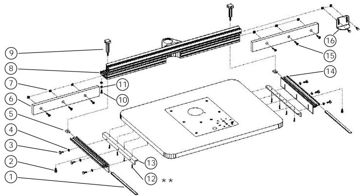
\*\* If you are mounting the Mast-R-Fence to a JessEm phenolic table top use the F0048 screws item (12A) listed below. We provide both these and wood screws which are supplied to be used for a custom table application.
