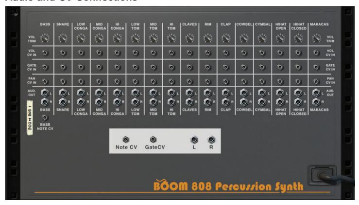
BOOM 808 has a variety of audio and CV connections to enable many creative options. In addition to main outputs and CV connections (shown by a white box), each instrument has its own individual connections available.
