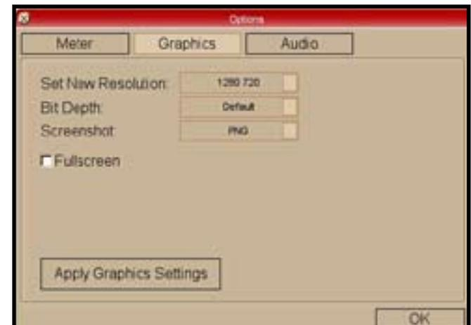
Again, placing your mouse over each item will activate a pop-up tag that explains what that item does. Changing the **Resolution** will change the shape and size of the VCM screen in the Windows “maximize” mode. (The VCM cannot be fully minimized.) **Fullscreen** will increase the screen size so that the VCM screen covers the Windows toolbars.
