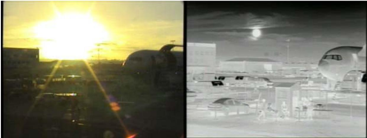
**Figure 7-1: Backlit daylight camera on left; thermal image on right**
