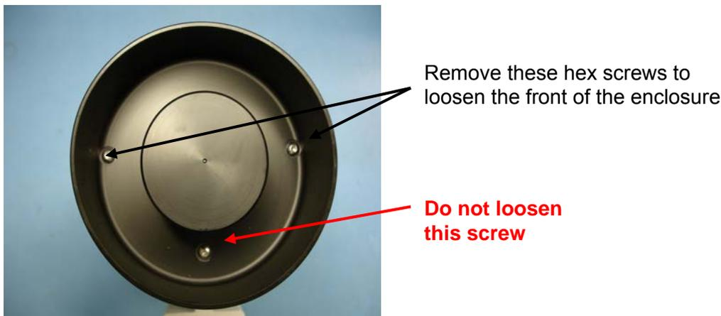
**Figure 6-1: Front view of SR-Series camera**
