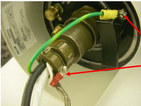
Cable shields from all cables (video, power, serial) are joined and connected to two ground leads (white and green) with terminal lugs.
