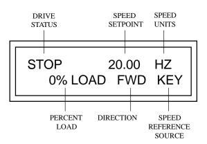
The display shown above indicates that the drive is stopped, the present speed setpoint is 20 Hz, there is no load (because it is stopped), the forward direction is selected, and the speed reference source is the keypad.
