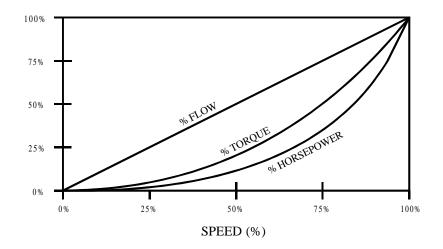
Variable torque refers to the fact that the torque required varies with the square of the speed. Also, the horsepower required varies with the cube of the speed, resulting in a large reduction in horsepower for even a small reduction in speed. It is easily seen that substantial energy savings can be achieved by reducing the speed of a fan or pump. For example, reducing the speed to 50% results in a 50 HP motor having to produce only 12.5% of rated horsepower, or 6.25 HP.
