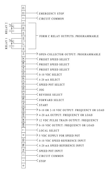
A complete description of operating the drive in the REMOTE mode can be found in Section 14.2. The following diagrams provide a quick reference for wiring the drive for the most common configurations.
