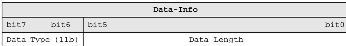
Data Type is fixed with 11b which meets "any other data" type of "Card Holder information" as MAD standard. And data length is including the data with ending zero "0", so the number of data byte sent by SmaFinger® is equal to data length with one less for RS232 output.
