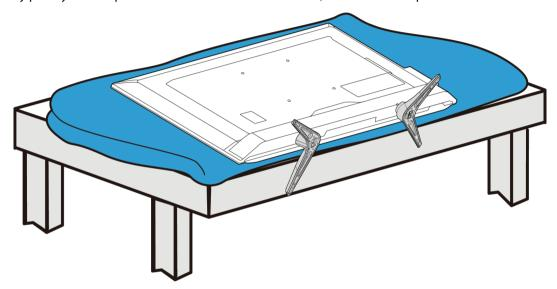
2 If the TV stands are installed, remove the four screws that secure the stands to your Sharp Roku TV.
