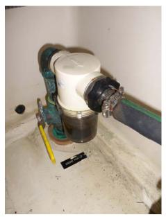
If upon restarting the engine overheats again, check the seal between the strainer, the rubber gasket, and the container. If the strainer is drawing air, it won't draw water. If needed, open and then retighten the lid on the strainer...and check to make sure the rubber gasket is in place in the lid (and not lying in the bilge.)
