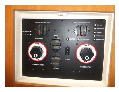
Battery voltage can be checked on the electrical panel. The starting battery is labeled "start" and the house battery is "house", a toggle switch changes the display to reflect what you are monitoring. You should try not to discharge below 11.5 volts before recharging the batteries by (1) running the diesel or (2) plugging into shore power. The charger is below the seat in the living room next to the kitchen.
