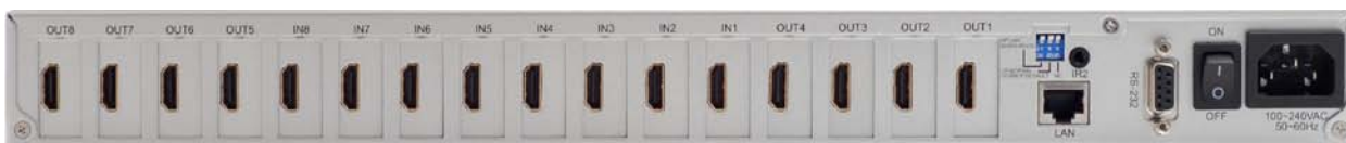
Figure 4-2 HDMI-8x8 Rear Panel
