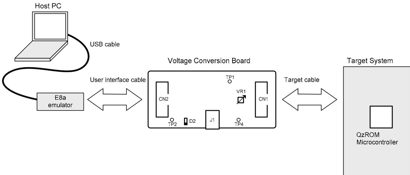
If you provide the power from the target system, or when you provide the VPP power from the power jack (J1) on the Voltage Conversion Board, please provide the power at this time.
