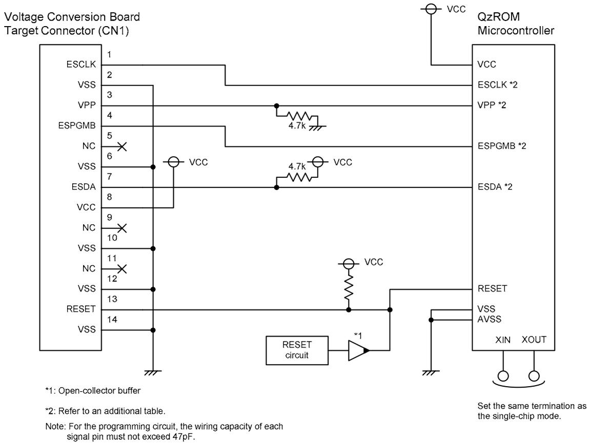
Figure 7-2 : Example of pin handling 2
