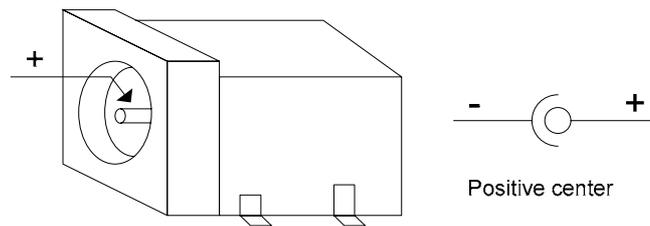
Figure 4-1: Power Jack (J1) Polarity
