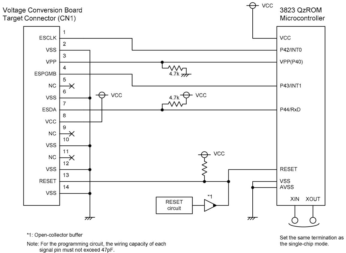
Figure 7-3 : Example of pin handling 3
