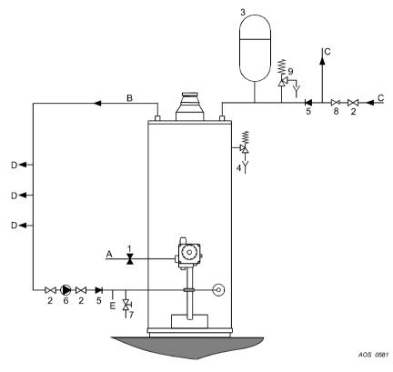
Figure 4 - Connection diagram (unvented system)
