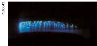
Fig. 3: diffuse vacuum arc AMF technology
