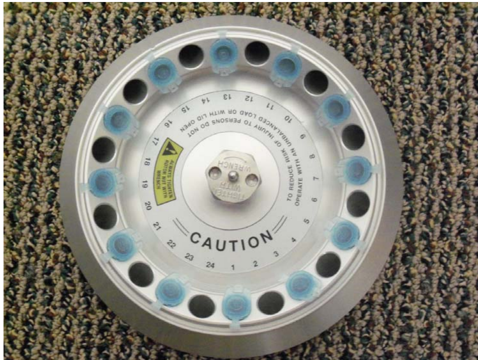
Figure 1. Loading the rotor to achieve balance
