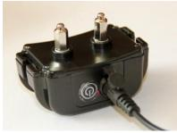
3) Power on the collar by holding the power button for 3 seconds. Install the rubber prongs if you have a small/medium size dog or the metal prongs if you have a medium/large dog.
