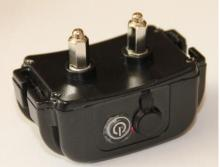
4) Test the shock of the collar by using the wire shock tester. Wrap the wires around the 2 metal posts of the collar then press the shock button. The bulb will light up if the collar is giving a shock.
