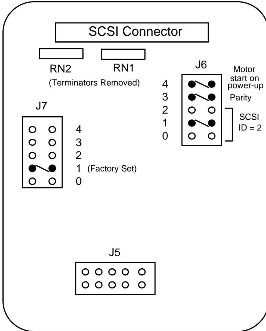
Figure B.6 - Maxtor MXT-1240S Hard Disk
