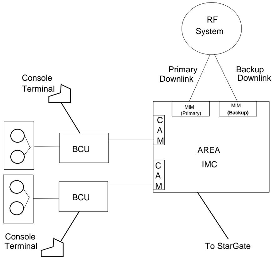
**Figure C.1 - EDACS Billing Fault Tolerant Architecture**
